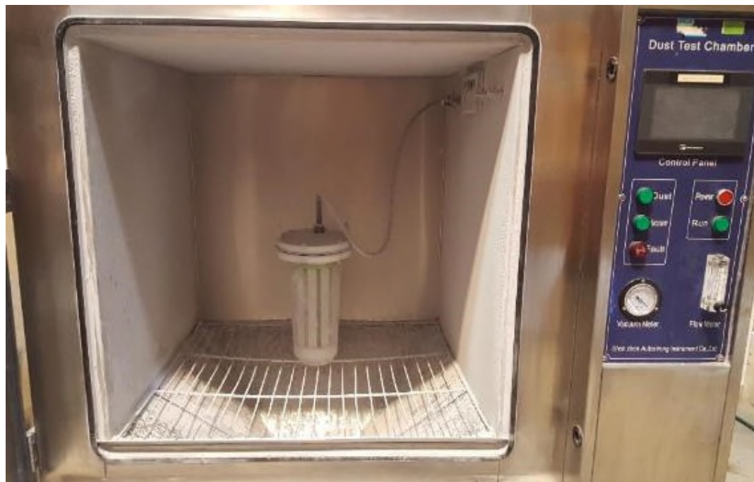
Figure 8: Product IP6X After Dust Test view.
