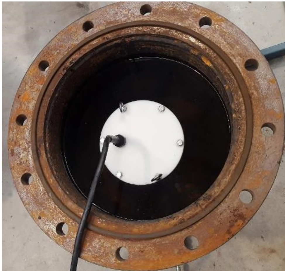
Figure 12: Product IPX8 Water Test Setup view.
