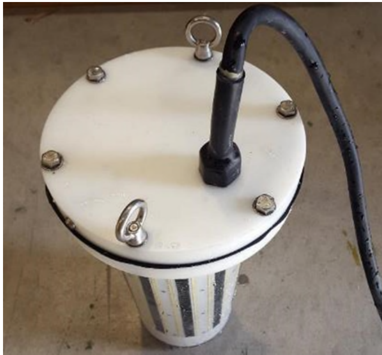
Figure 13: Product IPX8 After Water Test view.
