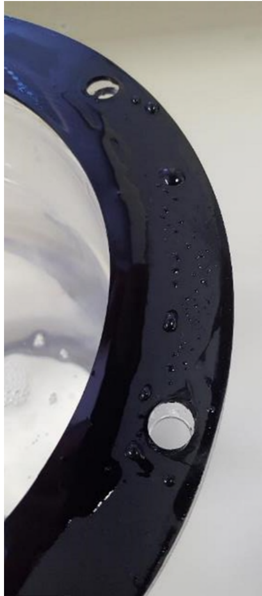
Figure 15: Product IPX8 After Water Test Inspection (Transformer fluid on inside, water droplets around middle) view.
