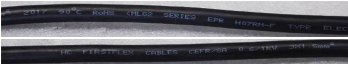
Figure 5: Product Power Cord Marking view.
