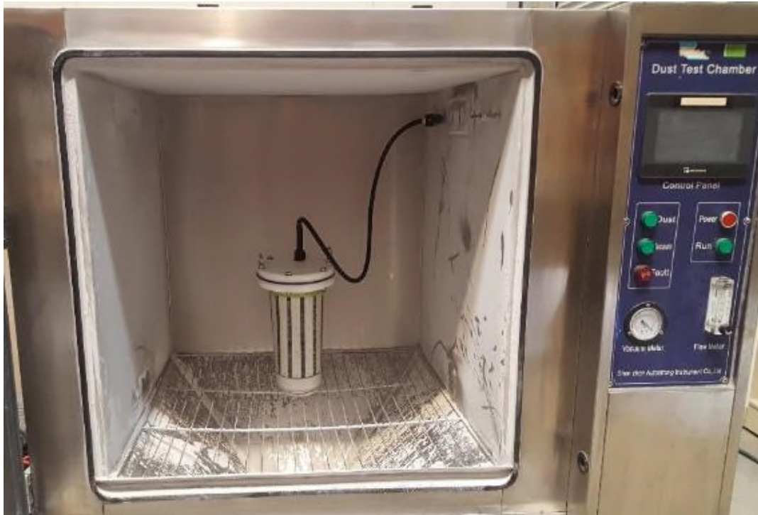
Figure 7: Product IP6X Dust Test Setup view.
