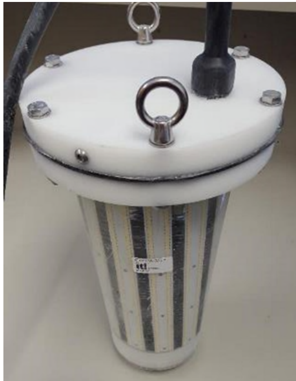
Figure 9: Product IP6X After Dust Test Inspection view.
