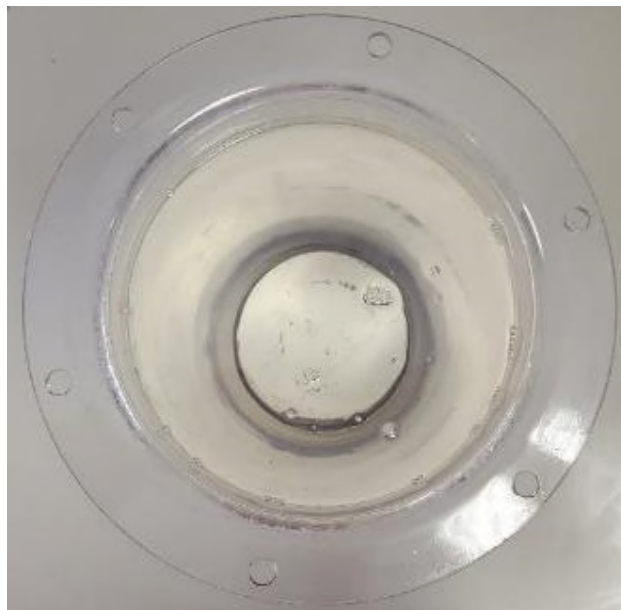
Figure 10: Product IP6X After Dust Test Inspection view.
